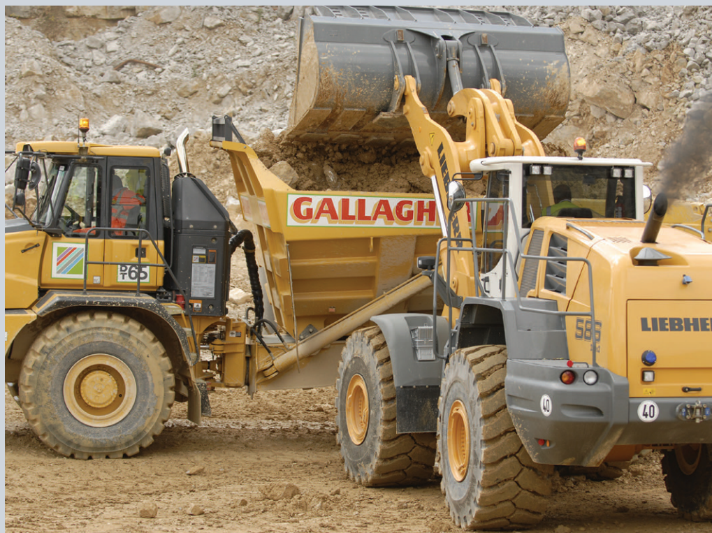
Figure 6 | The performance of hydraulic fluids in off-highway equipment has benefited greatly from the use of VI improvers. (Courtesy of The Lubrizol Corp.)
